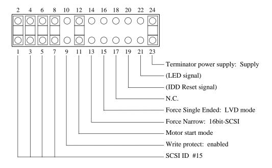
Figure 5.3 Setting terminals (CN2 on MP model only)
